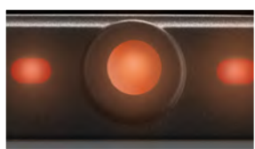
RPM and Temperature alarm leds
